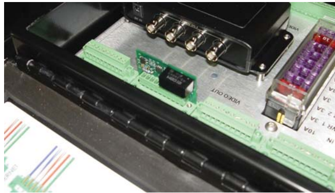
Figure 2: Bulkhead box JCU connection with NMEA card installed in Slot 3
