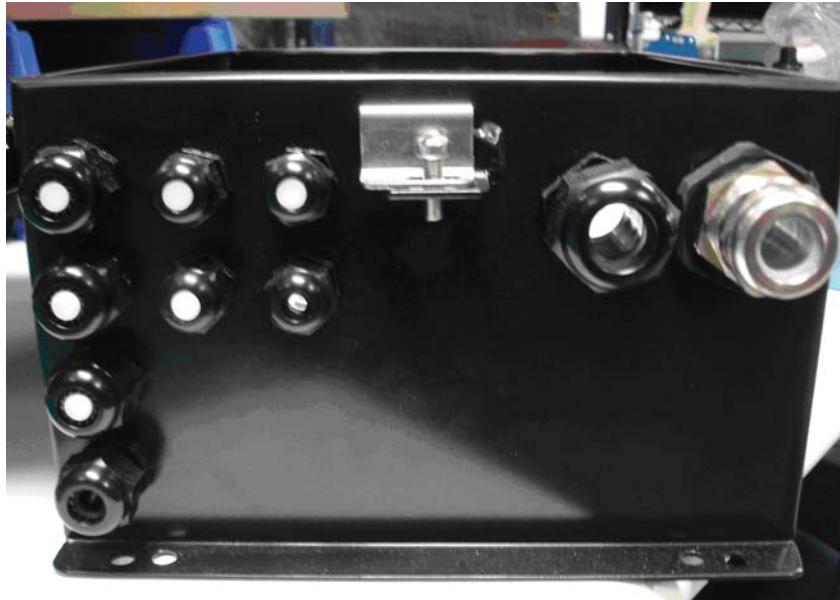
Figure 3: Cable Glands on the Bulkhead Box
