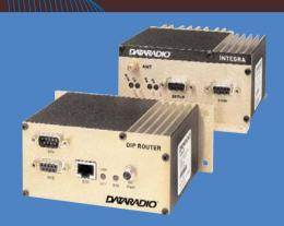
Our new Dataradio Private Wireless IP Gateway optimizes IP communications for transmission over your narrowband radio frequency. The optimized connectivity allows you to pass your critical SCADA information over an Ethernet connection back to your IP-based network. Each Private Wireless IP Gateway comes with the built-in flexibility of two distinct modes of operation:
