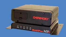
The Dataradio MobilPac II is a rugged, factory integrated, vehicular radio modem product designed to provide optimum data transmission performance for demanding mobile data applications. MobilPac II incorporates state-of-the-art Dataradio technology in a cost-effective, easy-to-install package. MobilPac II uses advanced DSP (digital signal processing) for high performance 19.2 Kbps and 14.4 Kbps operation.
