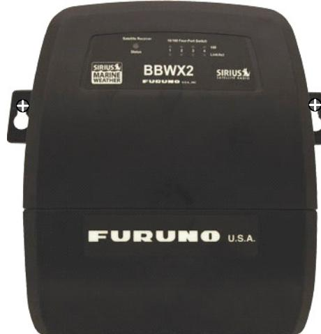
**Note:** The Antenna and **Receiver/Switch** should be mounted away from electromagnetic interference (e.g. >1.5 meters away from an AIS or radio transmitter, >2.0 meters away from Radar, >1.8 meters from a compass).
