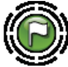
MOB mark on radar display
