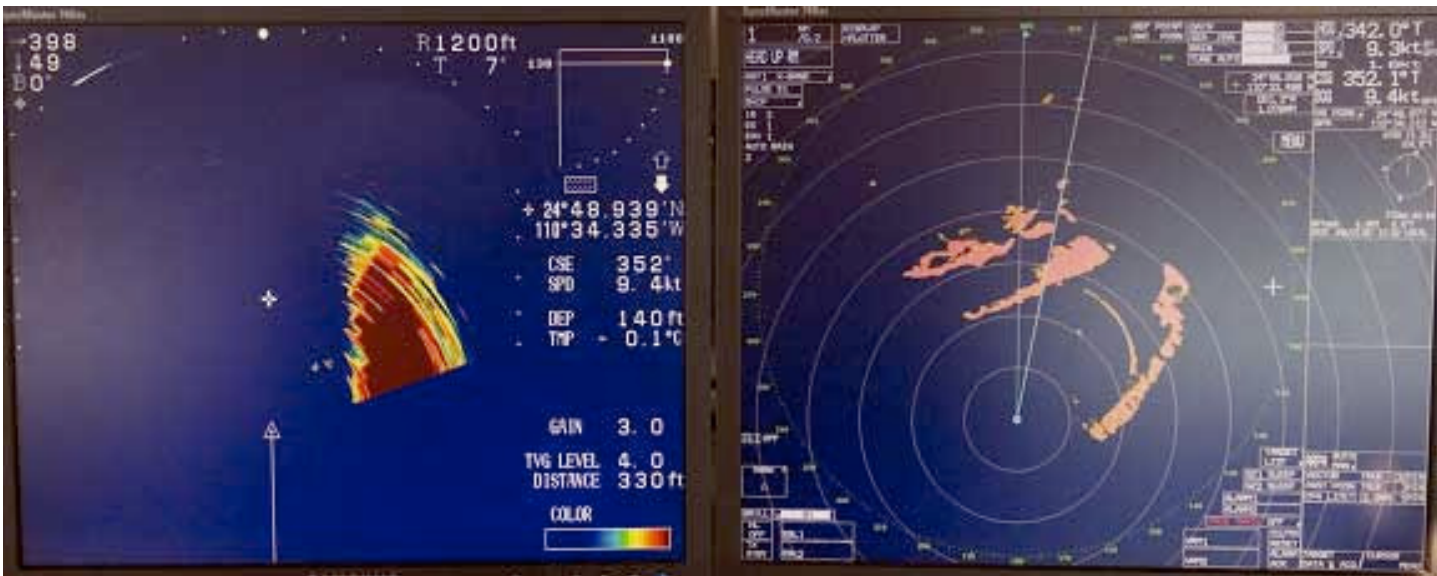
Putting the SONAR to work, here we are closing with the anchorage from the south. The SONAR (image above and left) is showing a clear path ahead, but there is something near the surface off our starboard bow (the dense red image). The RADAR screen on the right will put this into perspective. If you refer back to the Google image, you can see the hooked reef which is attached to the southern end of the island. That is giving us the SONAR return. Notice that this reef does not show up on radar as it is below the surface at high tide and it is also missing from the chart.
