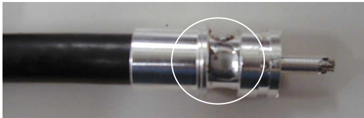
Solder shortage (No solder between the shield and connector)
