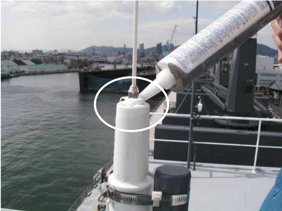
Fig. 3-16 Waterproofing of whip antenna base
