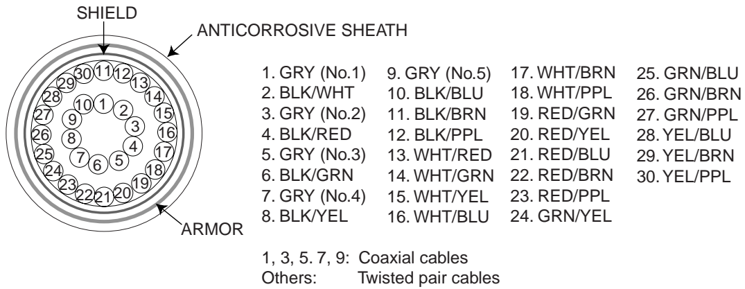
Cable 10S2074, sectional view
