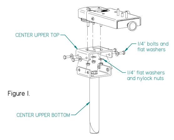
Attaching a DS-Clevis to the Mongoose Locking Slide Arm 7160-0119:
