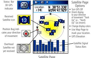
Displays your location coordinates, position accuracy, a view of the satellites overhead, and bar graph showing the signal strength of each overhead satellite.
