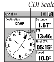
Navigation Page with Course Pointer and Course Deviation Indicator (CDI) Scale active.
