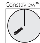
True Trails Constaview™ refreshes the image every 16ms. Despite heading changes trails are always true.
