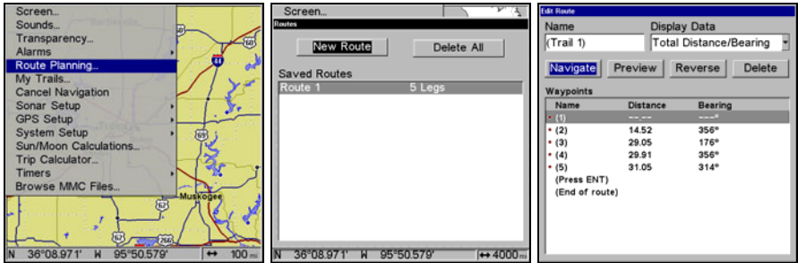
Route Planning on Main Menu (left). Routes menu (center). Edit Route menu (right). Navigate is selected on Edit Route menu.
