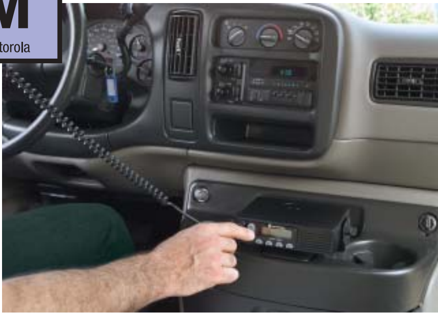
The Low-Profile Mounting Bracket keeps radio tucked up under the dash.
