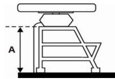
If the trestle height (A) is more than 2 m high, install a radar mast secured with guy wires as shown:
