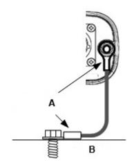
The eyelets must be crimped or soldered at both locations (A) and the method of connection to the vessel's hull is shown at (B).
