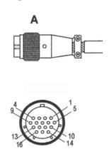
The interconnection cable pin details are provided here for information, in case the connector needs to be removed to feed the cable, or in case the cable needs to be shortened.
