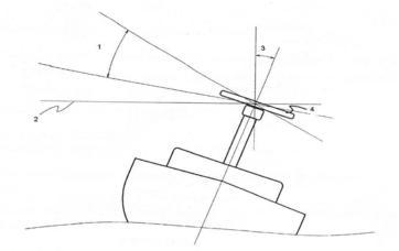
In this case, you're recommended to install the scanner on a gimbal mounting so that it can operate effectively in a heavy swell or when the yacht is heeled over.
