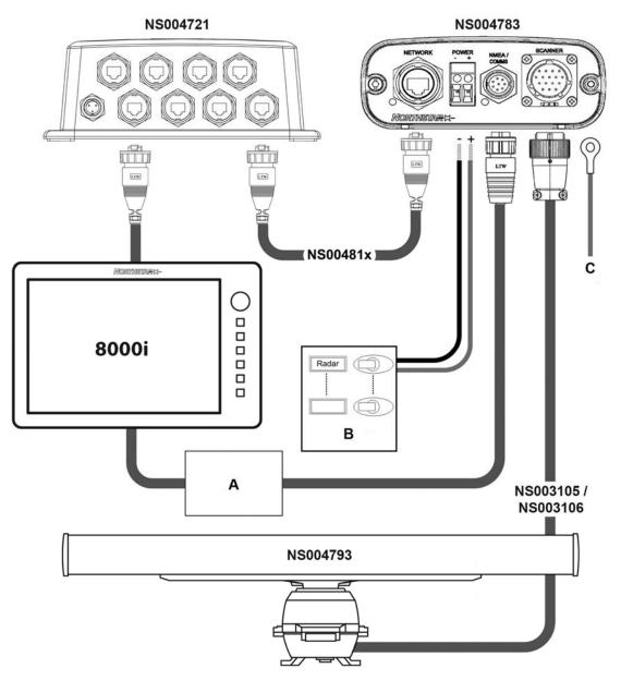
Configure the remote power control for an 8000i
