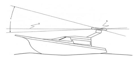
In this case, you're recommended to install the scanner so that is tilted down at the front, at an angle that will produce an almost horizontal sweep when the power boat is running at speed.
