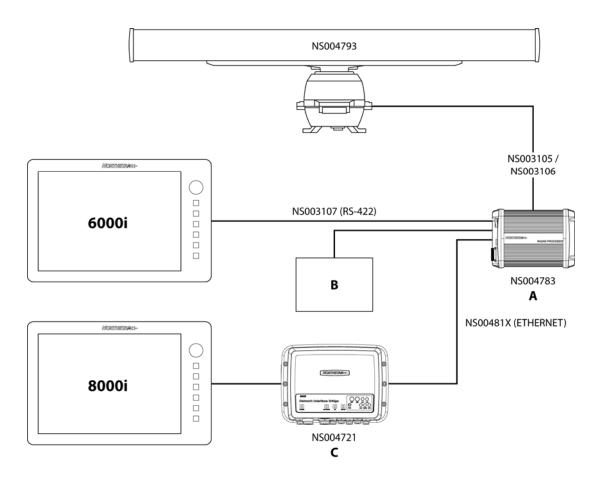
where A is the radar processor, B is the vessel's power supply (24 V DC ONLY), and C is the Network Linker (NS004721).
