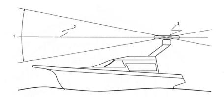
However, when the power boat is traveling at high speed, the bow rises up out of the water and if the elevation angle (trim) of the bow is raised up so that it equals, or exceeds, 50% of the vertical beam width of the radar, this can cause two problems:
