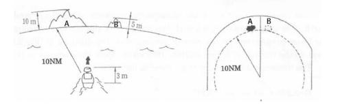
In this example, the scanner is installed on the vessel at a height of 10 ft (3 m) above sea level (h1). Island A is 33 ft (10 m) high (h2) and for comparison, Island B is 16.4 ft (5 m) high (h2). Both islands are at a distance (D) of 10 nautical miles from the vessel.
