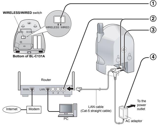
BL-C131A only: Confirm that the WIRELESS/WIRED switch on the bottom of the camera is set to WIRED.
