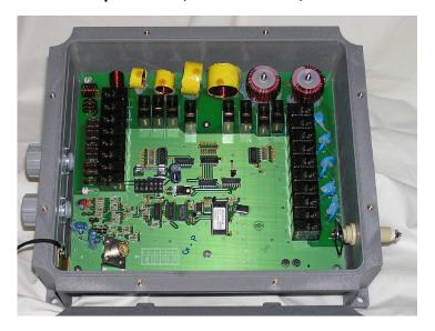
Designed and built by SEA, one of the industry's leaders in high technology, the SEA 1612C automatic tuner combines the sophistication of advanced microprocessor techniques with high order practicality and operational reliability. The SEA 1612C is housed in a weatherproof molded case designed to withstand the environmental conditions encountered aboard ship when mounted on the weather decks.
