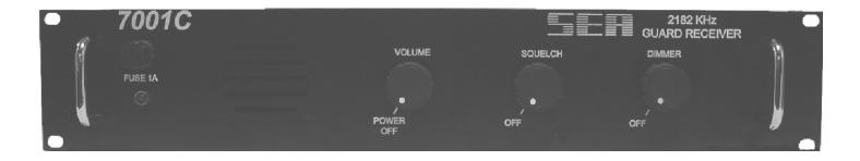
The SEA 7001C is a single channel, crystal controlled MF SSB receiver designed for watch-keeping applications on the International Distress and Calling frequency of 2182.0 kHz. It features high sensitivity and a mechanical filter with steep skirts to assure reception of important distress and emergency traffic. A voice-activated squelch circuit can mute the receiver when no signal is present and can be adjusted or disabled from the front panel.
