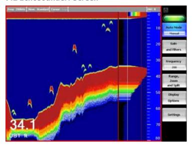
The *Echosounder* pane shows each echo as a vertical line of pixels. The echoes can be returned from 50 kHz only, from 200 kHz only, or from both of these frequencies mixed together.
