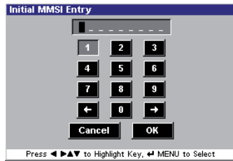
Figure 5.6 – MMSI Entry display
