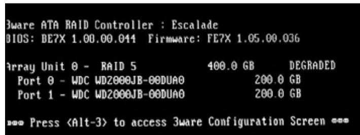
Figure 9.5: This is the BIOS screen for the 3ware controller. When you see it, type ‘Alt-3’ to enter the BIOS menu.
