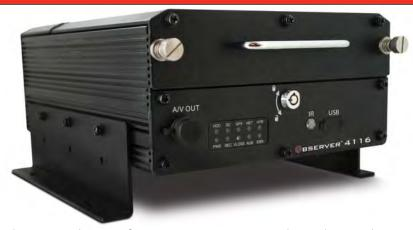
The Observer™ 4116 provides comprehensive features in a compact package designed to withstand the harsh vibrations and shock of the mobile environment. Using H.264 compression, up to 16 camera channels, complete with metadata, provides a complete mobile surveillance solution. Dual hard drives store up to 4 terabytes of data while a removable SD card duplicates, or mirrors, recorded events.
